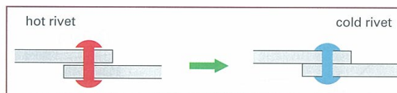
Figure 10.10 Joining two metal plates using a rivet.
