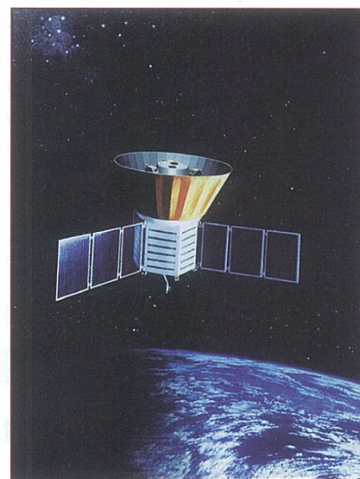
An artist's impression of the Cosmic Background Explorer. This spacecraft measured the temperature of space by detecting the radiation left over from the Big Bang. The gold-coloured 'skirt' shields the temperature sensors from heat from the Sun and Earth.
