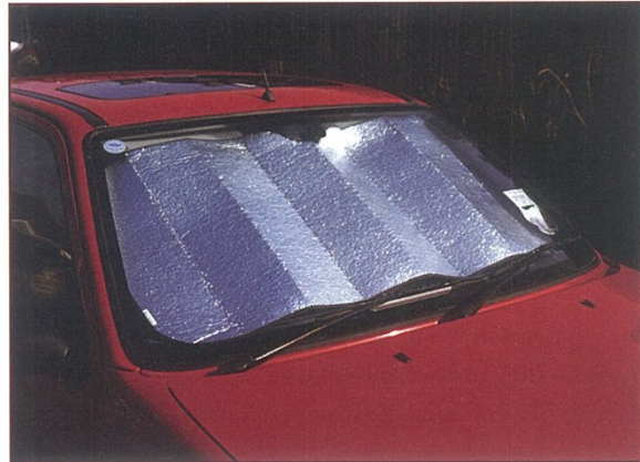
Figure 11.12 A sunshield reflects away unwanted radiation, which would otherwise make the car unbearably hot.
