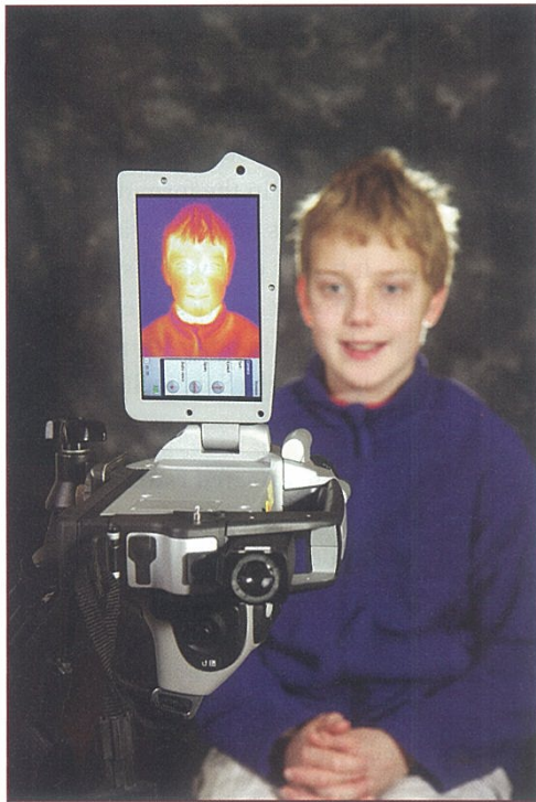
Figure 11.11 Using an infrared-sensitive camera. Slight variations in body temperature show up as different colours. Cameras like this are used in medicine to detect skin disorders and infections.
