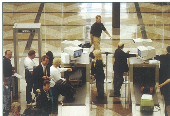
Figure 15.9 Two uses of electromagnetic radiation at the airport security check: X-rays are used to see inside the passengers' hand baggage, while radio waves detect metal objects as passengers walk through the arch.
