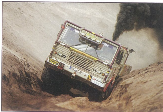
Figure 5.10 This truck has wide tyres to spread its weight as it travels over the sand dunes. Camels have big, flat feet for the same reason, to reduce the pressure on the sand so that they are less likely to sink in and become bogged down.
