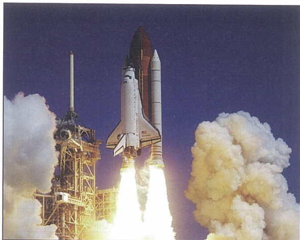
Figure 3.2 The space shuttle accelerating away from its launch pad. The force needed is provided by several rockets. Once each rocket has used all its fuel, it will be jettisoned, to reduce the mass that is being carried up into space.
