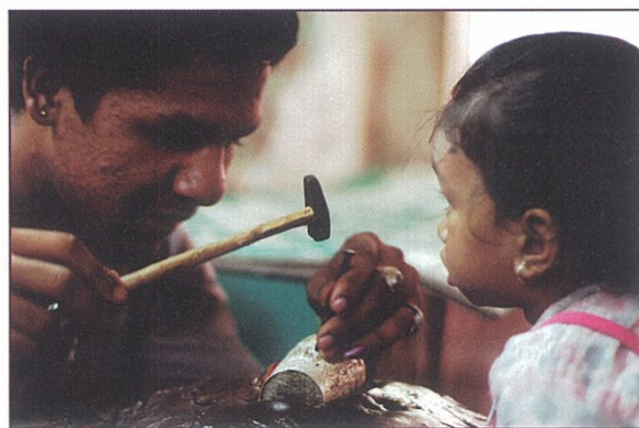
Figure 5.3 A Tibetan silversmith making a wrist band. Silver is a relatively soft metal at room temperature, so it can be hammered into shape without the need for heating.
